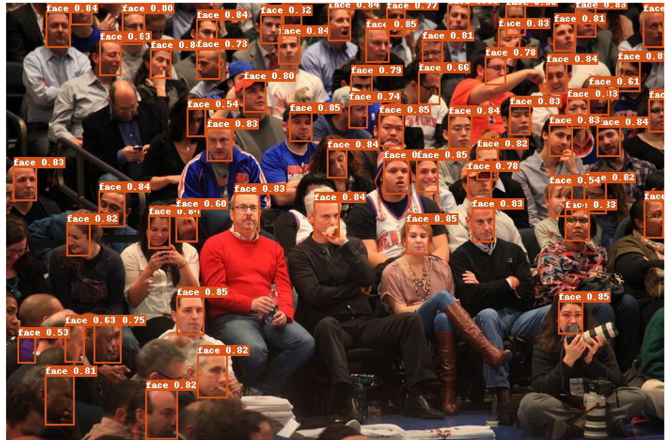
Fig. 8 UAV target detection effects. Our network successfully detects the faces of the vast majority of viewers in the figure, and the undetected faces lack features. They can be directly ignored in real applications
